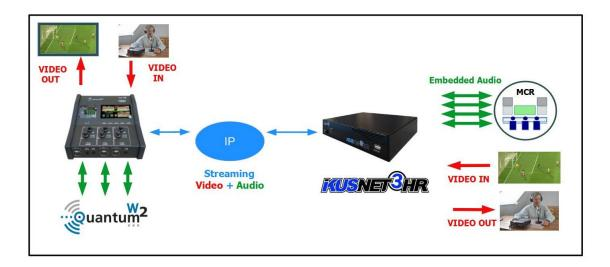
It is also possible to use the talkback channel to establish an audio connection between the Ikusnet3 HR and the Quantum2 laptop. This channel is independent of the video stream.
