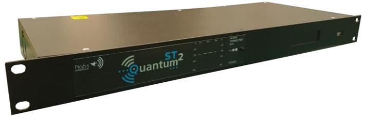
Double Ethernet and bonded LTE/5G support (optional together with HG2 product) are provided for wide area network connections.
